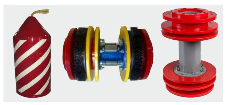
Pig is an equipment to clean pipeline. The outer edge of pig is elastically sealed to the inner wall of pipeline. Using gas, liquid or pipeline transport medium as the power source, the pig in the pipeline is pushed forward to the end of pipeline or the pig receiver.
